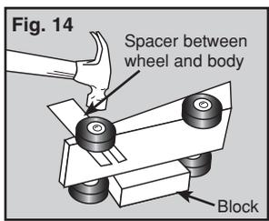
After installing Axles, check for toe-in/toe-out with your Wheel Alignment Tool or cardboard spacer. Toe-in or toe-out will slow the speed of your racer. You want your wheels aligned straight and parallel.
