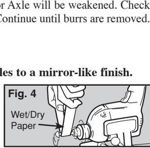
Next, mix a small amount of Pumice with water until it reaches an oatmeal-like consistency. Place a drop of the Pumice mixture in the center of a 1/4" x 4 1/2" strip of soft cloth. Run drill at medium speed and pass strip back and forth on Axle shank until it shines. Wash Axles in warm soapy water. Rinse and let dry. Repeat for each Axle.
