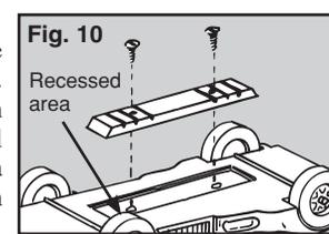
of the racer (**Fig. 10**). Weights may also be glued in place.
